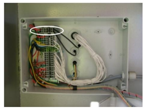
1. Remove the two blocks circled in the picture above, if fitted.
